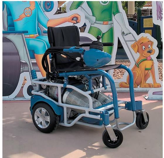
Figure 2. PneuChair prototype.
